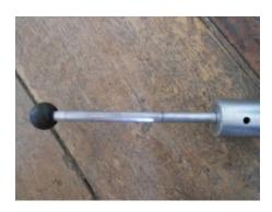
8) Make sure the **10 cm mark** in permanent marker is clearly depicted on compaction hammer. If not, measure 10 cm from the bottom of the hammer handle and make a new mark.
