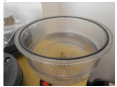
3) Make sure **O-ring** is correctly in place on bottom half of vacuum desiccator.
